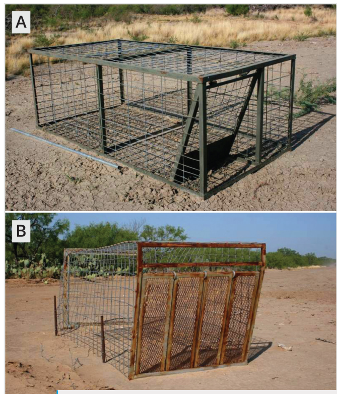
Figure 1. Box traps vary in size and construction. A common design includes a 4- by 8-foot cage built with durable materials (A). The best box traps are both effective and low cost. Many box traps are built from materials at hand (B).
