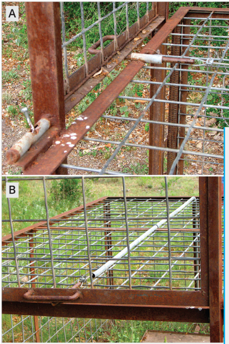
Figure 2. Many drop gates use a pin or similar object attached to a cable to hold the trap gate open (A). The cable can be slid through a conduit to the back of the trap, where it is attached to a trigger system (B). Trigger systems vary in design. (Source: Terry Gallagher)
